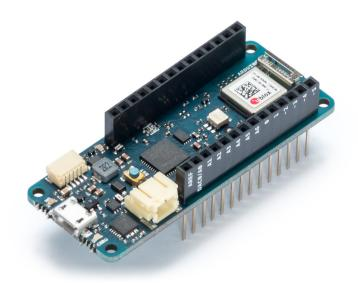
The MKR WIFI 1010 is a significant improvement on the MKR 1000 WIFI. It's equipped with an ESP32 module made by U-BLOX. This board aims to speed up and simplify the prototyping of WiFi based IoT applications thanks to the flexibility of the ESP32 module and its low power consumption.
