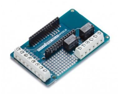
The MKR Relay Shield allows you to easily add relays to your MKR board based project.
