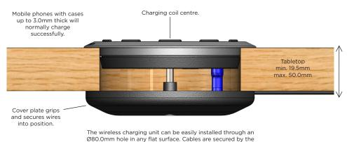
retaining plates completing the installation.
