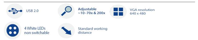
In addition, the series offers video frame rates up to 30 fps and the ability to save files in BMP, JPG and AVI format. Professional-quality imaging results can be viewed on any computer via high speed USB 2.0 output and the included DinoCapture (for PC) or DinoXcope (for MAC) software. The Dino-Lite AM2111 Basic is an excellent choice for hobbyists, schools, kids or any other cost sensitive application.
