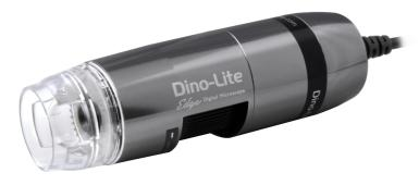
The AM7515MT4A is a 5MP Dino-Lite Edge Series microscope that has a magnification range of 415x - 470x with built-in coaxial illumination. By using the Flexible LED Control (FLC), this model is capable of switching between or mixing, brightfield and coaxial illumination.
