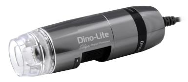
The AM7515MT8A is a 5MP Dino-Lite Edge Series microscope that has a magnification range of 700-900x with built-in coaxial illumination. By using the Flexible LED Control (FLC), this model is capable of switching between or mixing, brightfield and coaxial illumination.
