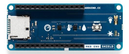
To help you build projects and store the data collected locally, this shield has a slot for a microSD card (not provided).
