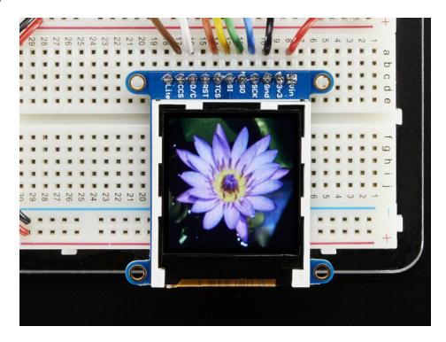
This lovely little display breakout is the best way to add a small, colorful and bright display to any project. Since the display uses 4-wire SPI to communicate and has its own pixel-addressable frame buffer, it can be used with every kind of microcontroller. Even a very small one with low memory and few pins available!
