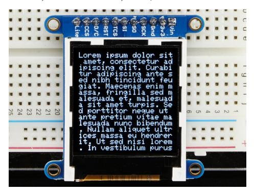
The 1.44" display has 128x128 color pixels. Unlike the low cost "Nokia 6110" and similar LCD displays, which are CSTN type and thus have poor color and slow refresh, this display is a true TFT! The TFT driver (ST7735R) can display full 16-bit color using our library code.
