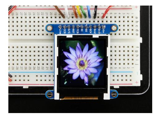
To make new bitmaps, make sure they are less than 128 by 128 pixels and save them in **24-bit BMP format!** They must be in 24-bit format, even if they are not 24-bit color as that is the easiest format for the Arduino. You can rotate images using the **setRotation()** procedure
