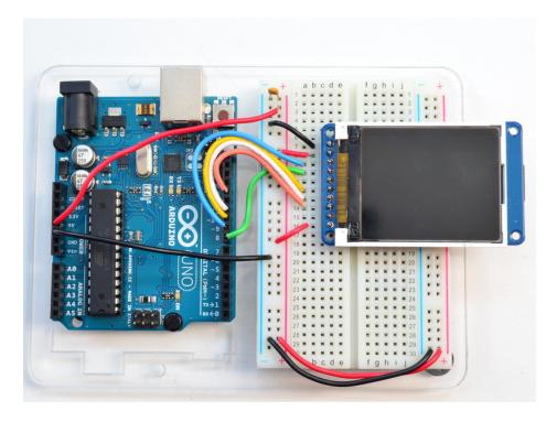
Wiring up the display in SPI mode is pretty easy as there's not that many pins! We'll be using hardware SPI, but you can also use software SPI (any pins) later. Start by connecting the power pins
