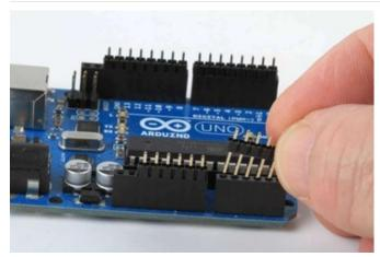
Insert the Headers into an Arduino To align the header strips for soldering, insert them (long pins down) into the headers of an Arduino.
