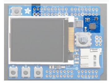
Instead of taking up a bunch of GPIO pins to read the buttons and joystick, as well as controlling the TFT backlight, we use an I2C expander chip called the seesaw. It is connected to the SDA/SCL pins and can read/write pins with our library. This saves a ton of pins and then you can always use the I2C pins for other sensors, as long as the address doesnt conflict
