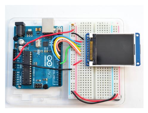
Once you are sure that the TFT is wired correctly, add the two wires for talking to the SD card. Connect **CARD\_CS** (the unconnected pin in the middle) to digital pin **4** (you can change this later to any pin you want). Connect **MISO** (second
