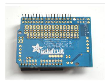
Start by sliding the 10 pin,  $2 \times 8$  pin and 6-pin stacking headers into the outer rows of the shield from the top. Then flip the board over so its resting on the four headers. Pull on the legs if necessary to straighten them out.
