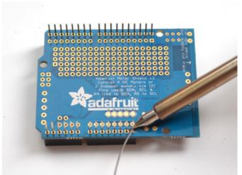
Tack one pin of each header, to get them set in place before more soldering. If the headers go crooked you can re-heat the one pin while re-positioning to straighten them up
