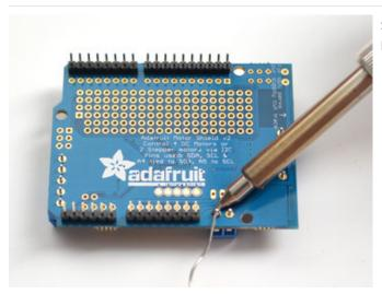
Solder in the two pins of the external power terminal-block
