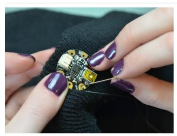
You can start with the pixel + or -. For this hat we chose to start with the shared ground line that hooks up all the sequins. Stitch around the GND pad on GEMMA at the edge of a knit cap and knot/seal at the back.
