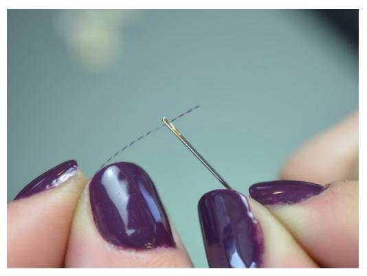
Grab a needle and test it's small enough to pass through the holes in the sequins. Thread up your needle with conductive thread, our 2-ply and 3-ply both are great for this purpose. Check out our conductive thread guide to learn more about this stainless steel fiber.
