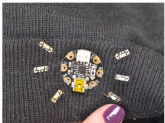
Next hook up the + connections from each of GEMMA's outputs to three pixels. We stitched from one sequin to the GEMMA, then over to another sequin and on to the third sequin before going back to the first, making a sort of square that results in the thread tails being in the same place.
