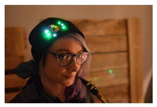
You can make the LEDs fade and twinkle by using the PWM (a.k.a. analogWrite) functionality of your Gemma or Flora, or just connect directly to a digital I/O pin of a microcontroller to turn on and off (digitalWrite).
