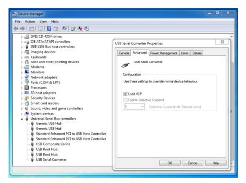
Now unplug and plug in again the FT232H board and check device manager again to find the USB Serial Port (COMx) node in the Ports (COM & LPT) node. That's it, you're all set to access the device as a serial COM port in Windows!
