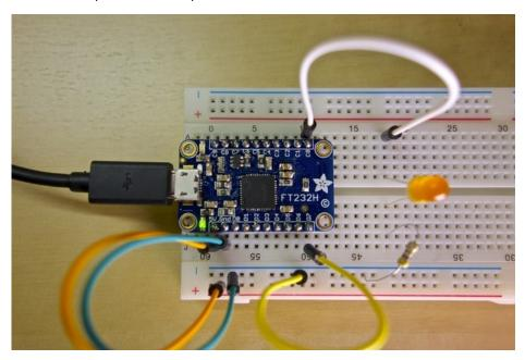
With this configuration pin **C0** will be a digital output that controls if the LED is on or off, depending on the level of the **C0** output. Pin **D7** will be a digital input that reads if it's at a high level (3-5 volts) or low level (ground).
