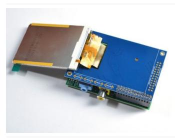
Before attaching the display, check that all the pins are soldered nicely and there's no bridging, cold solder, shorts, or unsoldered pins.
