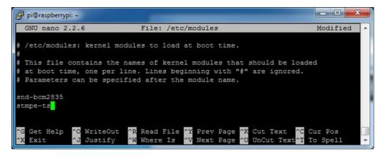
Save the file and reboot the Pi with sudo reboot and look at the console output (or rundmesg in the console window
