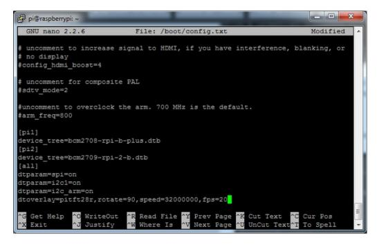
The rotate= variable tells the driver to rotate the screen 0 90 180 or 270 degrees.
