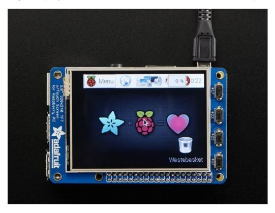
In order to add support for the 2.4" or 2.8" TFT and touchscreen, we'll need to install a new Linux Kernel. Lucky for you, we created a kernel package that you can simply install *over* your current Raspbian (or Raspbian-derived) install instead of needing a whole new image. This makes it easier to keep your install up-to-date.
