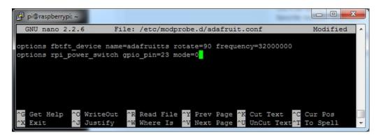
To make it active immediately run sudo modprobe rpi\_power\_switch
