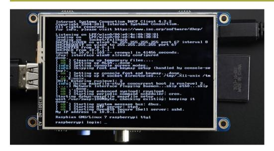
One fun thing you can do with the display is have it as your main console instead of the HDMI/TV output. Even though it is small, with a good font you can get 20 x 40 of text. For more details, check out <a href="https://github.com/notro/fbtft/wiki/Boot-console">https://github.com/notro/fbtft/wiki/Boot-console</a>
