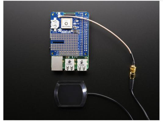
All Ultimate GPS modules have a built in patch antenna - this antenna provides -165 dBm sensitivity and is perfect for many projects. However, if you want to place your project in a box, it might not be possible to have the antenna pointing up, or it might be in a metal shield, or you may need more sensitivity. In these cases, you may want to use an external active antenna. (http://adafru.it/960)
