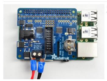
Plug the red wire into the + side, and the black wire into the - side.
