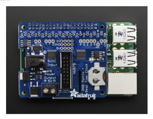
Each order comes with a HAT PCB with all surface mount parts assembled, a 2x20 female socket connector, a 2 pin terminal block, and a 2x8 IDC socket connector. A CR1220 coin cell is not included to make air shipping easier, please order one seperately (https://adafru.it/em8) if you do not have one and would like to use the real time clock.
