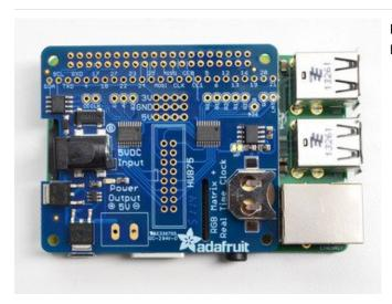
Place the HAT on top so that the short pins of the 2x20 header line up with the pads on the HAT
