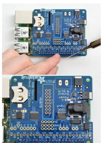
Check over your work so far, make sure each solder point is shiny, and isn't bridged or dull or cracked
