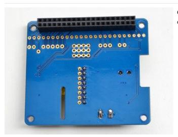
Check your work! Make sure all the solder points are clean and not shorted or cracked or dull
