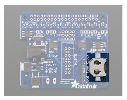
The rgb-matrix.sh script already installed the necessary software to use the realtime clock...but you'll need to set the initial time once. This is explained in the "Sync time from Pi to RTC" section of this DS1307 tutorial (https://adafru.it/IF1) (just that one section...you can ignore the rest).
