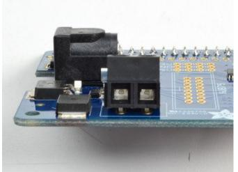
Place the 2 pin terminal block first, make sure the two 'mouths' are facing outwards
