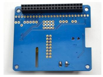
Flip the board over, the tape should keep the connector from falling out
