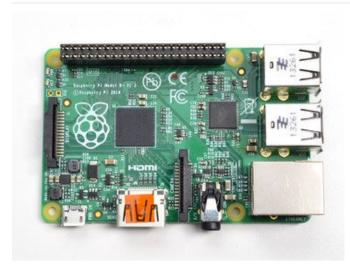
Start by plugging the 2x20 header into a Raspberry Pi, this will keep the header stable while you solder. Make sure the Pi is powered off!
