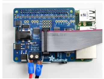
The RGB matrix also came with a 2x8 data cable. Connect one end to the matrix's INPUT side and the other end to the IDC socket on the HAT/bonnet.
