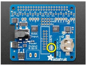
Look for the Address E pads located between the HUB75 connector and Pi camera cutout.
