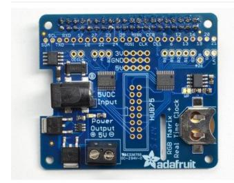
Next up we will attach the 2x8 IDC header. Unlike the 2x20 header, this connector has a direction!
