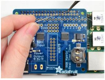
Flip the board around and solder all the connections for the other half of the 2x20 header
