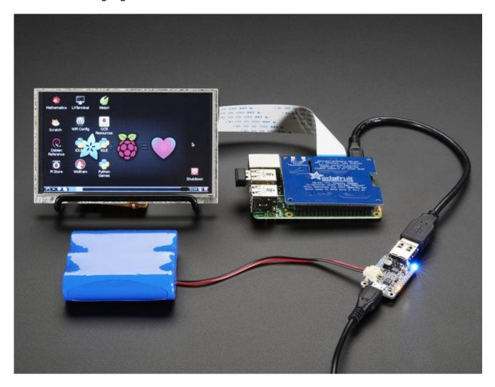
The PowerBoost 1000C has at the heart a <u>TPS61090 boost converter from II</u> (http://adafru.it/duQ). This boost converter chip has some really nice extras such as low battery detection, 2A internal switch, synchronous conversion, excellent efficiency, and 700KHz high-frequency operation. Check out these specs!
