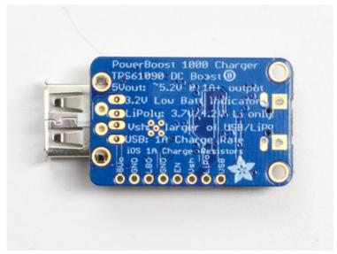
Snap the USB connector in so that all of the pins go through the PCB. Make sure you're solder them on the back of the PCB
