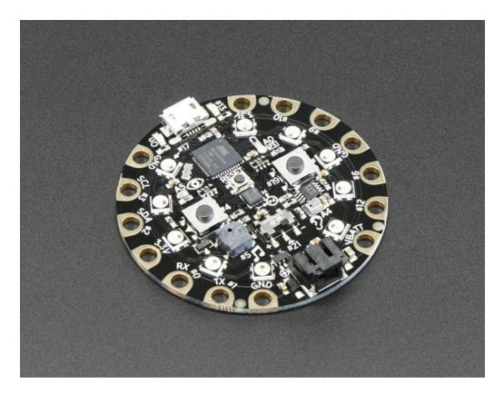
Circuit Playground has built-in USB support. Built in USB means you plug it in to program it, it just shows up - all you need is a Micro-B USB cable, no additional purchases are needed! With the new 1.6.4+ Arduino IDE, it takes only a few seconds to add support. The Circuit Playground has USB HID support, so it can act like a mouse or keyboard to attach directly to computers.
