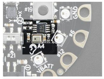
Microphone Audio Sensor A MEMS microphone can be used to detect audio levels and even perform basic FFT functions. You can read the analog voltage corresponding to the audio on analog pin #A4. Note that this is the raw analog audio waveform! When it's silent there will be a reading of ~330 and when loud the audio will read between 0 and 800 or so. Averaging and smoothing must be done to convert this to sound-pressure-level.
