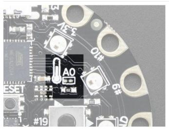
Temperature Sensor There is an NTC thermistor (Murata NCP15XH103F03RC) that we use for temperature sensing. While it isn't an all-in-one temperature sensor, with linear output, it's easy to calculate the temperature based on the analog voltage on analog pin #A0. There's a 10K resistor connected to it as a pull down.
