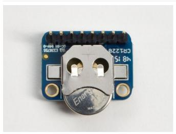
Don't forget that the Real Time Clock requires a battery backup. A CR1220 size battery goes in the back, make sure the + symbol on the battery is visible when you insert!
