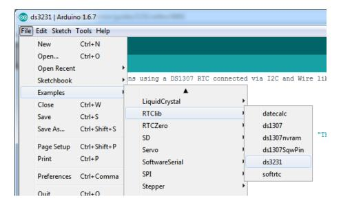
Upload to your Arduino and check the serial console @ 9600 baud. After a few seconds, you'll see the report that the Arduino noticed this is the first time the DS3231 has been powered up, and will set the time based on the Arduino sketch.
