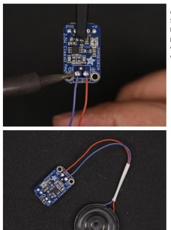
Connect Wires to Amp Secure the amp back onto the helping third hands. Solder the positive wire from the speaker to the positive output pin on the amp, then, solder the negative wire to the negative output pin. Now we can proceed to work on the power circuit.
