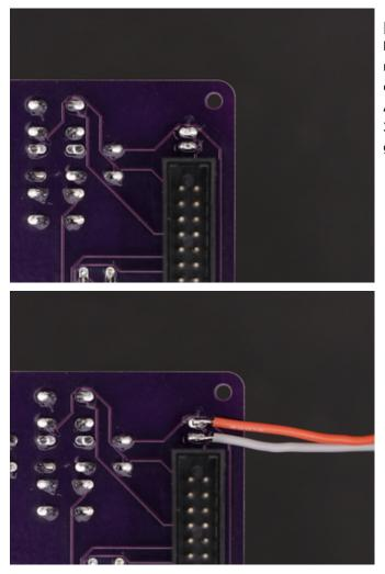
Prep Power Pins on Gamepad PCB Locate the power label on the gamepad PCB and take note of the **5V** and **GND** pins. Flip the gamepad PCB over and secure it to a Panavise to hold it in place. Apply solder to the two pins and solder in our two 26AWG wires. Use the photo to reference which wires goes were (red right, white left).
