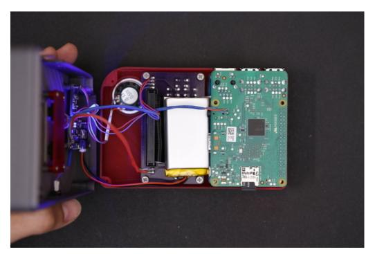
Once they're separated, reposition the battery and listen carefully to the noise. Position the battery in a spot where the noise is less prominent and mount it in place with tape or mounting tack.
