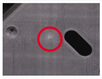
Be careful tapping the standoffs from the top -To prevent puncturing the surface, **DO NOT** tap all the way through the standoff. Be careful not to tap too fast or forcefully to avoid damaging the standoffs.
