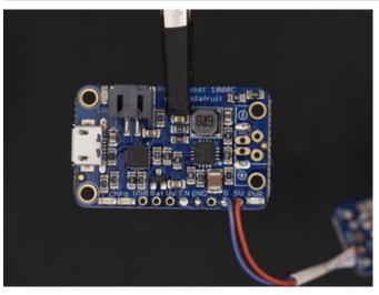
Connect Amp to PowerBoost 1000C Slip on a piece of heat shrink tubing to the wires connected to the Vin and Gnd pins. Next, secure the PowerBoost 1000C to the helping third hands. Solder the VIN wire from the amp to the 5V pin on the PowerBoost. Then, solder the Gnd wire from the amp to the G pin on the PowerBoost 1000C.
