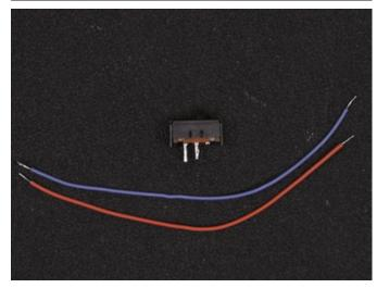
Prep Slide Switch Remove one of the legs from the slide switch. Secure the switch to the helping third hands and apply solder to the two remaining legs. Now we'll need two new 30AWG wires that measure abot 7cm in length. Strip and tin the tips of each wire.
