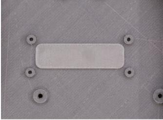
Shoulder Button (cont.) Fasten four #2-56 3/8 into the standoffs of the shoulder mount. Screw them in until the barely protrude the standoff - this is going to make it easier to mount it to the case. Next, insert the rubber shoulder button actuator into the cutout of the bottom case part.
