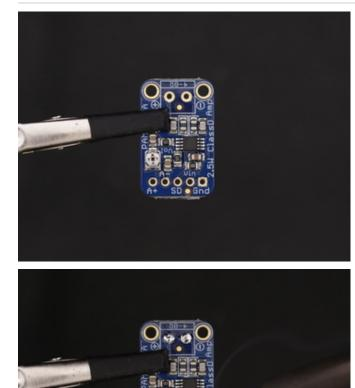
Prep PAM8302 Amp Secure the amp to a pair of helping third hands. Use the tip of the soldering iron to heat up solder and apply to the VIN, GND, A+, A–, + and – pins. This will make it easier to solder wires to the pins.
