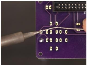
Solder Buttons to Gamepad PCB Secure the gamepad PCB to a Panavise and solder up the buttons. Make sure solder joints are clean like you did on the pins of the IC box header.
