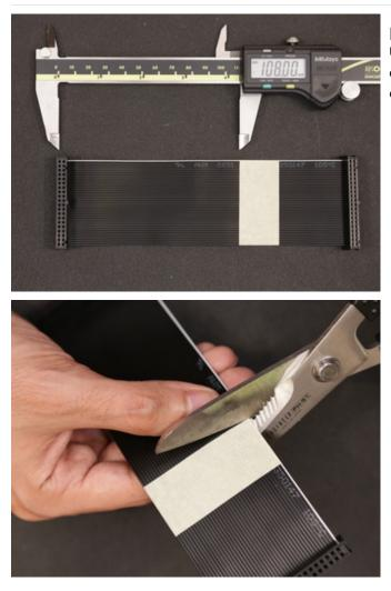
Measure, Mark and Cut Ribbon Cable Use a pair of calipers or measuring tape to get the desired length and mark the ribbon cable - Tape, marker or otherwise.
