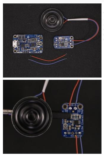
Measure Wires for PowerBoost and Amp We'll need about 3cm in length of 30AWG wire to connect the Amp to the PowerBoost 1000C. Use wire strippers to remove about 4mm of insulation from each tip and apply solder to tin them. Now secure the amp to the helping third hands and solder the wires to the **Vin** and **Gnd** pins.
