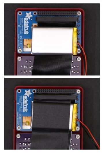
Install Lipo Battery Now we can install the 2000mAh lipo battery. A good spot for it is right behind the PiTFT display. To keep it in place, we can use a piece of gaffers tape. Try to keep it up closely against PiCable. Position it like in the photo, closer to the right side to avoid intersecting with some of the components from the Pi.
