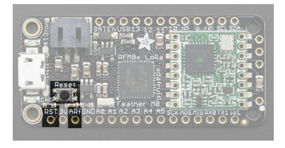
• RST - this is the Reset pin, tie to ground to manually reset the AVR, as well as launch the bootloader manually
