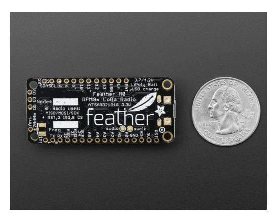
This **Feather MO LoRa Radio** uses the extra space left over to add an RFM9x LoRa 868/915 MHz radio module. These radios are not good for transmitting audio or video, but they do work quite well for small data packet transmission when you need more range than 2.4 GHz (BT, BLE, WiFi, ZigBee).
