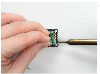
Strip a mm or two off the end of the wire, tin and solder into the **ANT** pad on the very right hand edge of the Feather
