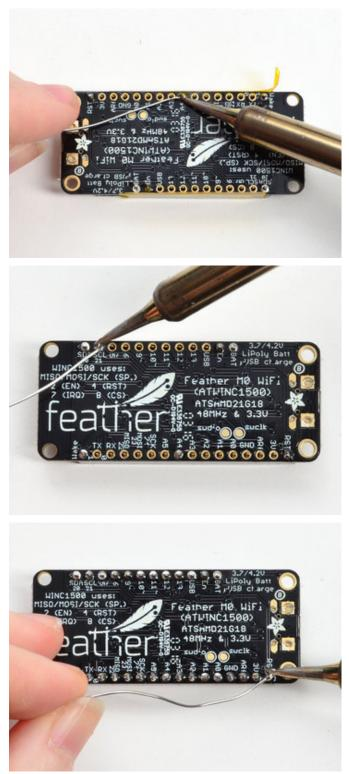
And Solder! Be sure to solder all pins for reliable electrical contact.
