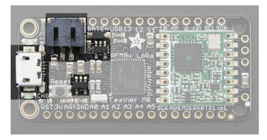
The above shows the Micro USB jack (left), Lipoly JST jack (top left), as well as the 3.3V regulator and changeover diode (just to the right of the JST jack) and the Lipoly charging circuitry (to the right of the Reset button). There's also a **CHG** LED, which will light up while the battery is charging. This LED might also flicker if the battery is not connected.
