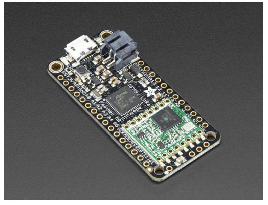
This is the Adafruit Feather MO RFM95 LoRa Radio (433 or 900 MHz) - our take on an microcontroller with a "Long Range (LoRa)" packet radio transceiver with built in USB and battery charging. Its an Adafruit Feather MO with a Long Range radio module cooked in! Great for making wireless networks that are more flexible than Bluetooth LE and without the high power requirements of WiFi. We have other boards in the Feather family, check'em out here.
