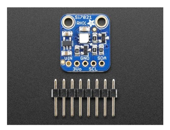
We put this nice sensor on a breakout board with a 3.3V regulator and level shifting so you can use it safely with 3.3V or 5V power & logic. There's a PTFE filter to keep the sensor clean, that's the white flat thing on top. Also comes with some pin header. Some light soldering is required to attach the header but it's easy to do.
