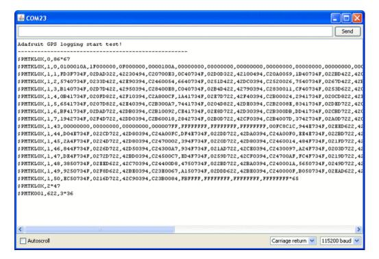
Copy and paste all the text after the —'s (starting with \$PMTKLOX,0,86\*67 and ending with \$PMTK001,622,3\*36) then paste it into the box located on this page
