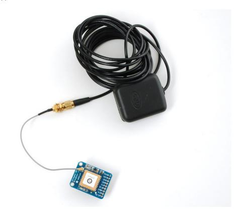
All Ultimate GPS modules have a built in patch antenna - this antenna provides -165 dBm sensitivity and is perfect for many projects. However, if you want to place your project in a box, it might not be possible to have the antenna pointing up, or it might be in a metal shield, or you may need more sensitivity. In these cases, you may want to use an external active antenna.
