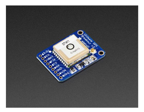
The breakout is built around the MTK3339 chipset, a no-nonsense, high-quality GPS module that can track up to 22 satellites on 66 channels, has an excellent high-sensitivity receiver (-165 dB tracking!), and a built in antenna. It can do up to 10 location updates a second for high speed, high sensitivity logging or tracking. Power usage is incredibly low, only 20 mA during navigation.
