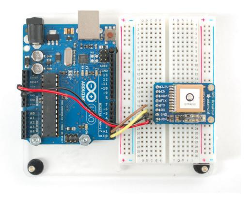
Now plug in the USB cable, and open up the serial monitor from the Arduino IDE and be sure to select **9600 baud** in the drop down. You should see text like the following:
