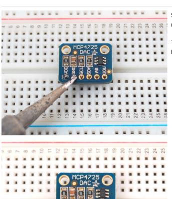
Solder each pin using a soldering iron and solder, to make solid connection on each pin.
