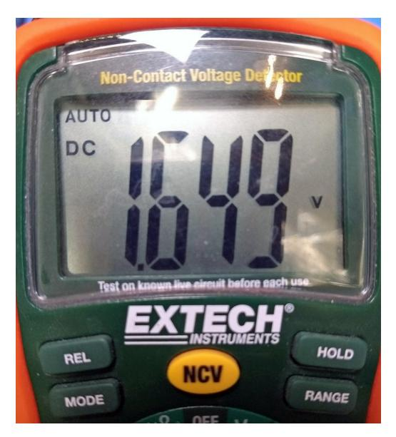
Hook up a multimeter to the **Vout** pin of the board (positive/red lead to **Vout**, ground/black lead to board GND) and you should see about 1.65 volts DC output. Try setting **dac.value** to other numbers like 0 or 65535 to see how the voltage changes.
