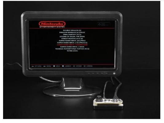
First, install the micro SD card into the Raspberry Pi Zero. Then, plug in the HDMI cable to a monitor or TV. You will need to use the mini HDMI side of the cable on the Raspberry Pi Zero, and the full size HDMI for your TV or monitor. Now, use the included power adapter and plug it in to the 'PWR IN' port on the Raspberry Pi Zero.
