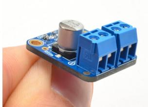
Next we will solder in the two 3.5mm terminal blocks used to connect power & the motor to the breakout board.
