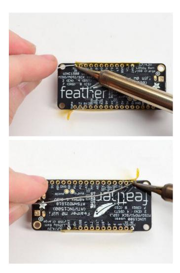
And Solder! Be sure to solder all pins for reliable electrical contact.
