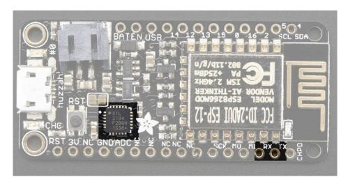
The **TX** pin is the output *from* the module and is 3.3V logic.
