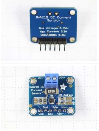
Wires can be soldered directly to the holes on the edge of the board. But for breadboard use, you will want to solder on the included 6-pin header.
