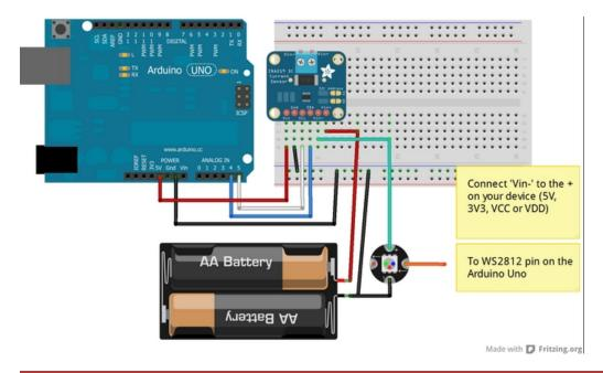
Be careful inserting noisy loads that can cause a sharp current draw, such as DC motors, since they can cause problems on the power lines and may cause the INA219 to reset, etc. When using a DC motor or a similar device, be sure to include a large capacitor to decouple the motor from the power supply and use a snubber diode to protect against inductive spikes.
