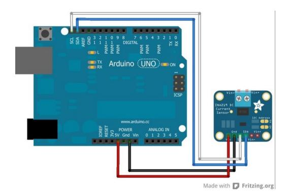
Next we must insert the INA219 current sensor into the circuit we want to measure:
