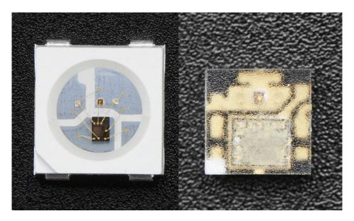
The first example will show you how to change the color and brightness of the internal RGB LED.
