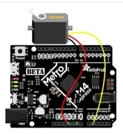
For the Metro M4 Express, ItsyBitsy M4 Express and the Feather M4 Express, connect the ground wire to any G or GND, the power wire to USB or 5V, and the signal wire to A1.
