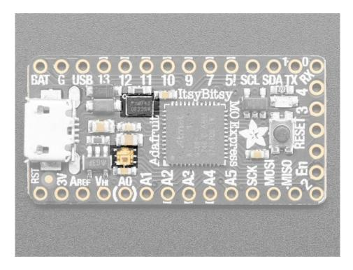
The **DotStar** is connected to pin #40 (clock) and #41 (data) in Arduino, so just use our DotStar library (https://adafru.it/zbD) and set it up as a single-LED strand on pins 40 & 41. The DotStar is powered by the 3.3V power supply but that hasn't shown to make a big difference in brightness or color. The DotStar is also used by the bootloader to let you know if the device has enumerated correctly (green) or USB failure (red). In CircuitPython, the LED is used to indicate the runtime status.
