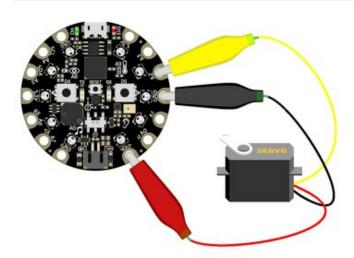
For Circuit Playground Express, use jumper wire alligator clips to connect the ground wire to GND, the power wire to VOUT, and the signal wire to A2.
