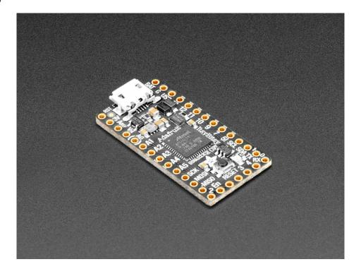
What's smaller than a Feather but larger than a Trinket? It's an **Adafruit ItsyBitsy MO Express!** Small, powerful, with a rockin' ATSAMD21 Cortex MO processor running at 48 MHz - this microcontroller board is perfect when you want something very compact, but still with a bunch of pins.
