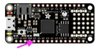
A0 is located between GND and A1 on the opposite side of the board from the battery connector, towards the end with the Reset button.
