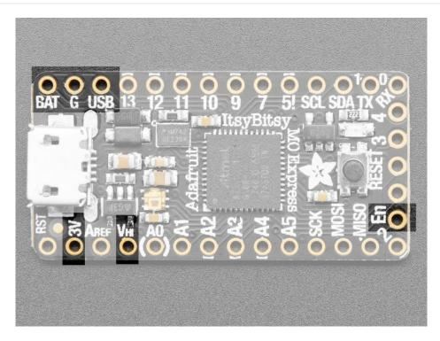
The ItsyBitsy M0 Express has  ${\bf BAT} \; {\bf G} \; {\bf USB} \; {\bf on} \; {\bf the} \; {\bf top} \; {\bf left}, \; {\bf right} \; {\bf next} \; {\bf to} \; {\bf the} \; {\bf micro} \; {\bf USB} \; {\bf port}$
