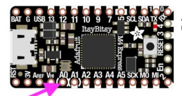
A0 is located between VHI and A1, and the pin pad has left and right white parenthesis markings around it.
