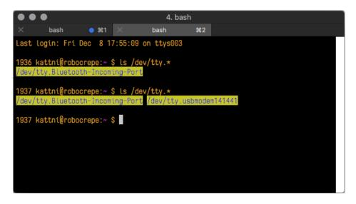
Using Mac, a new listing has appeared called /dev/tty.usbmodem141441 . The tty.usbmodem141441 part of this listing is the name the example board is using. Yours will be called something similar.
