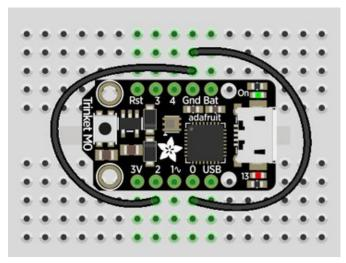
This wiring example shows A1 and A2 connected to ground.
