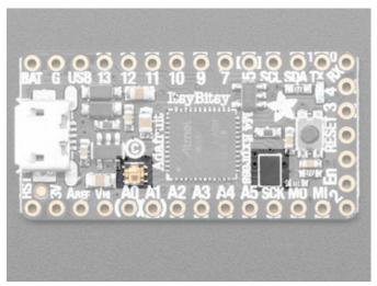
As part of the 'Express' series of boards, this ItsyBitsy is designed for use with CircuitPython. To make that easy, we have added two extra parts: a mini DotStar (RGB LED) and a 2 MB QSPI (Quad SPI) Flash chip
