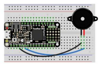
Use jumper wires to attach A1 and one of the two GND to different legs of the piezo.
