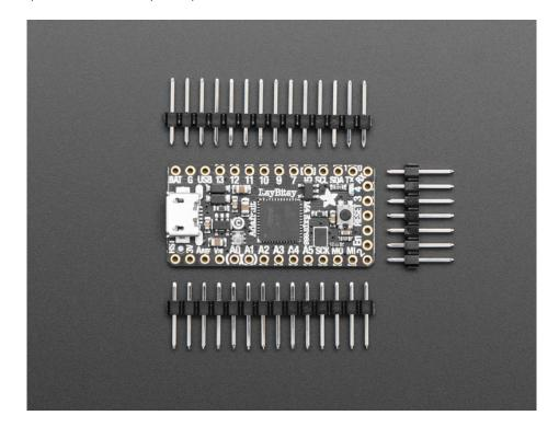
Each order comes with one assembled and tested ItsyBitsy M4, with headers that can be soldered in for use with a breadboard. ItsyBitsy M4 comes with CircuitPython programmed in, but you can replace the code with Arduino if you like.
