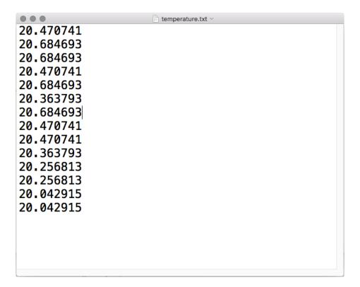
This file gets updated once per second, but you won't see data come in live. Instead, when you're ready to grab the data, eject and unplug your board. For CPX, move the switch to the left, otherwise remove the wire connecting the pin to ground. Now it will be possible for you to write to the filesystem from your computer again, but it will not be logging data.
