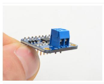
Now you can do the terminal block, this is what you'll use to attach the thermocouple since you cannot solder to thermocouples
