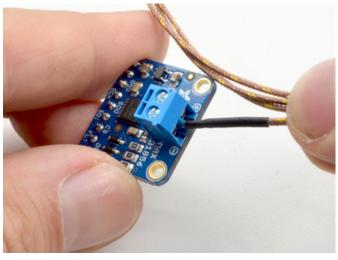
Insert the thermocouple wires and tighten down the clamps with a small Phillips or flat screwdriver
