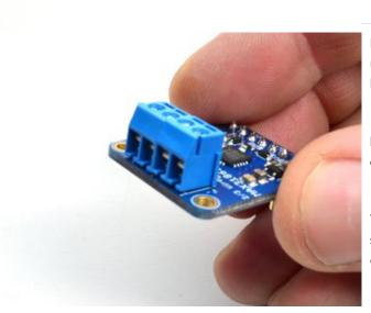
Next we will solder in the two 3.5mm terminal blocks used to connect power & the motor to the breakout board.
