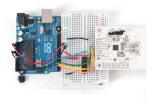
Also, we need to select SPI as the interface so on **SEL1** place the jumper in the **ON** position. for **SEL0** place the jumper in the **OFF** position.
