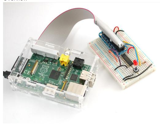
Now that you've finally got your hands on a Raspberry Pi® (https://adafru.it/aHx), you're probably itching to make some fun embedded computer projects with it. What you need is an add on prototyping Pi Cobbler from Adafruit, which can break out all those tasty power, GPIO, I2C and SPI pins from the 26 pin header onto a solderless breadboard. This mini kit will make "cobbling together" prototypes with the Pi super easy.
