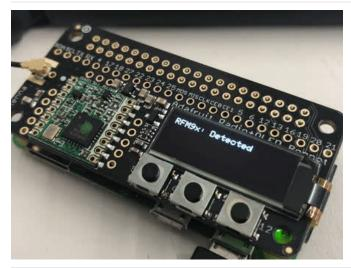
If the RFM9x/RFM69 is **detected**, the OLED will display **Detected**. You can test the buttons by pressing them.
