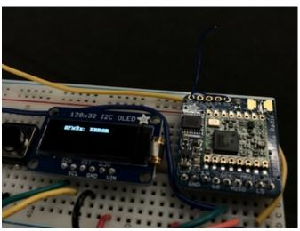
If the wiring of the radio module is incorrect - the display will show ERROR. Check over your wiring on the Wiring Page and re-run the test. You may also need to ensure the correct CircuitPython library is installed for the module.
