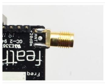
Use plenty of solder to make sure you have a good strong mechanical connection. The duck antennas are long and make great levers, so they could pry apart the solder joints if not soldered well
