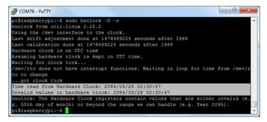
You can see, the date at first is invalid! You can set the correct time easily. First run date to verify the time is correct. Plug in Ethernet or WiFi to let the Pi sync the right time from the Internet. Once that's done, run **sudo hwclock -w** to write the time, and another **sudo hwclock -r** to read the time
