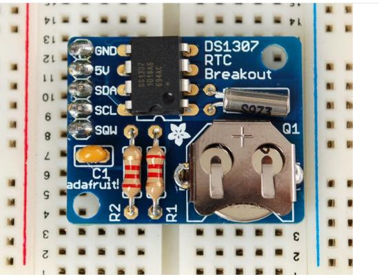
This tutorial requires a Raspberry Pi running a kernel with the RTC module and DS1307 module included. Current Raspbian distros have this, but others may not!
