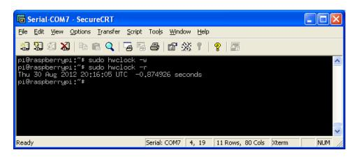
Next, you'll want to add the RTC kernel module to the /etc/modules list, so its loaded when the machine boots. Run sudo nano /etc/modules and add rtc-ds1307 at the end of the file (the image below says rtc-1307 but its a typo)
