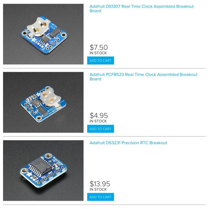
Don't forget to also install a CR1220 coin cell. In particular the DS1307 wont work at all without it and none of the RTCs will keep time when the Pi is off and no coin battery is in place.
