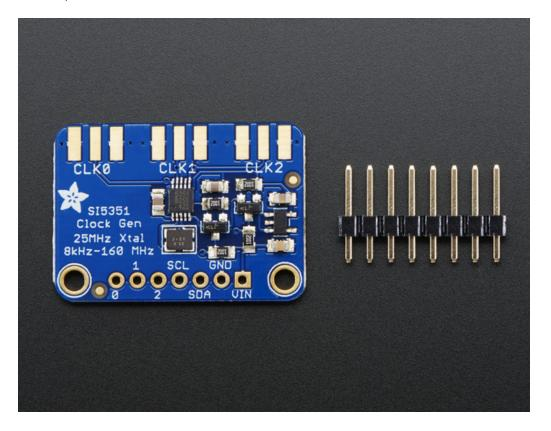
The Si5351 clock generator is an I2C controller clock generator. It uses the onboard precision clock to drive multiple PLL's and clock dividers using I2C instructions. By setting up the PLL and dividers you can create precise and arbitrary frequencies. There are three independent outputs, and each one can have a different frequency. Outputs are 3Vpp, either through a breadboard-friendly header or, for RF work, an optional SMA connector.
