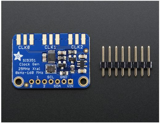
If you have the breadboard version of this sensor, you'll want to solder some header onto the sensor so it can be used in a breadboard.
