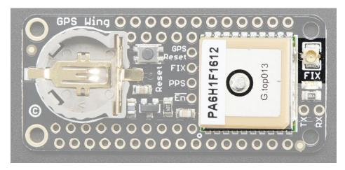
All Ultimate GPS modules have a built in patch antenna - this antenna provides -165 dBm sensitivity and is perfect for many projects. However, if you want to place your project in a box, it might not be possible to have the antenna pointing up, or it might be in a metal shield, or you may need more sensitivity. In these cases, you may want to use an external active antenna. (http://adafru.it/960)
