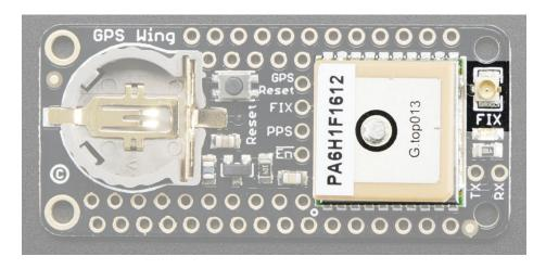
You have two options for an antenna. The GPS module has an antenna on it already, that's the square tan ceramic thing on the left side. If you plug an *active GPS antenna* into the uFL connector on the very right, the module will automatically switch over to the external antenna.
