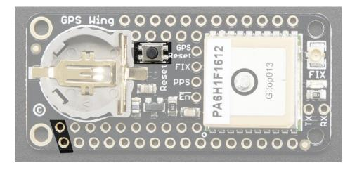
There is a small button that will connect the *microcontroller* RESET pin to ground for resetting it. Handy to restart the Feather. Note that this is not connected to GPS reset unless you short the jumper on the back!
