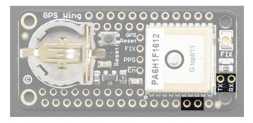
The GPS module, like pretty much all GPS's, communicates over UART serial. It sends ASCII NMEA setences from the
