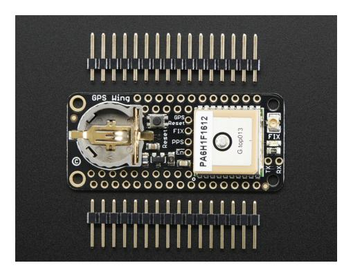
Comes as a fully assembled FeatherWing with GPS module and a coin cell holder. However, the 12mm coin cell is**not included** - it isn't required but if you would like a battery backup, a CR1220 coin battery must be purchased seperately. We also toss in some header so you can solder it in and plug into your Feather
