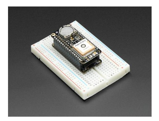
The Wing is built around the MTK3339 chipset, a no-nonsense, high-quality GPS module that can track up to 22 satellites on 66 channels, has an excellent high-sensitivity receiver (-165 dB tracking!), and a built in antenna. It can do up to 10 location updates a second for high speed, high sensitivity logging or tracking. Power usage is incredibly low, only 20 mA during navigation.
