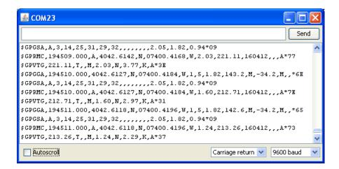
Look for the line that says \$GPRMC,194509.000,A,4042.6142,N,07400.4168,W,2.03,221.11,160412,,,A\*77 This line is called the RMC (Recommended Minimum) sentence and has pretty much all of the most useful data. Each chunk of data is separated by a comma.
