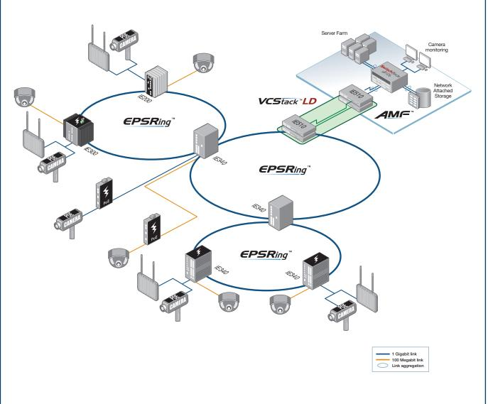
EPSRing<sup>™</sup> and ITU-T G.8032 provide high-speed resilient ring connectivity. This diagram shows the IE Series in a double ring network topology.
