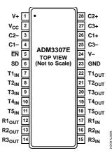
Figure 5. SSOP/TSSOP Pin Configuration
