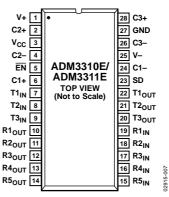
Figure 7. SSOP/TSSOP Pin Configuration
