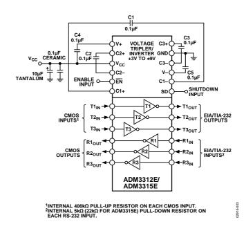
Figure 3. ADM3312E/ADM3315E Functional Block Diagram
