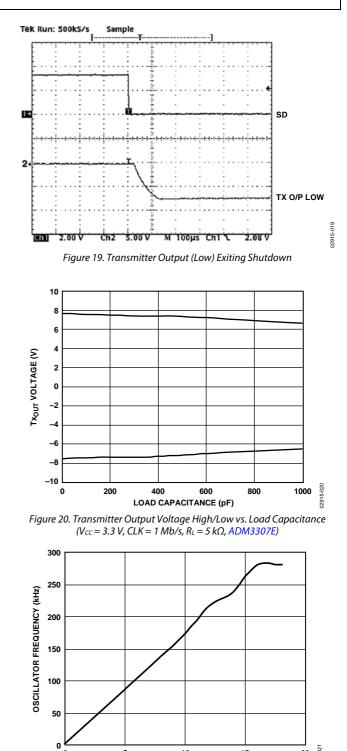
10 LOAD CURRENT (mA) Figure 21. Oscillator Frequency vs. Load Current
