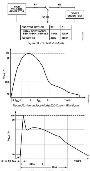
Figure 36. IEC1000-4-2 ESD Current Waveform
