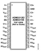
Figure 9. SSOP/TSSOP Pin Configuration
