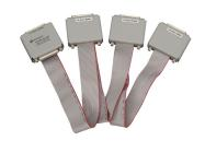
This adapter is required to use the multiple units of the B2901A/02A/11A/12A with EasyEXPERT group+ software. The adapter has 4 Dsub25 connectors, which enables you to connect up to 4 units of the B2901A/02A/11A/12A and to control them through EasyEXPERT group+software.
