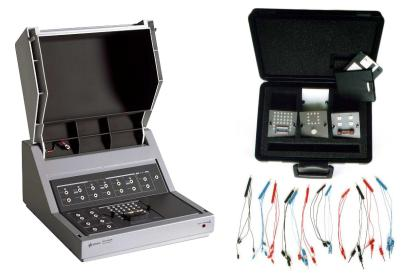
The 16442B Test Fixture can also be used with the B2900A Series Precision Instruments. The 16442B Test Fixture has 6 triaxial connectors and 6 BNC coaxial connectors for interfacing with the B2900A Series Precision Instruments. The triaxial connectors of the 16442B support up to 200 V and 1 A DC. It is compatible with the B2901A/02A/11A/12A and B2961A/62A.
