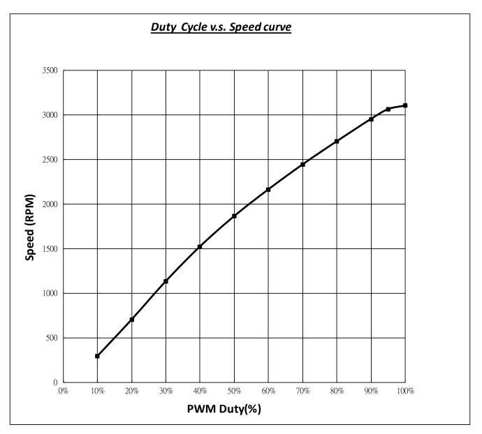
NOTE: It is tested under free air condition. The same spec is not able to apply in static pressure condition
