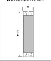
Fig. 22-5 Hole pattern for wall mounting
