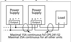
Fig. 12-2 Using distribution terminals
