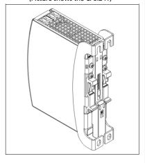
Fig. 22-4 **Wall/panel mounting, front view** (Picture shows the CP5.241)
