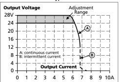
Fig. 6-2 **Dynamic output current capability, typ.**
