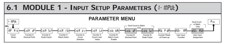
Shaded area selections only apply when Counter B is enabled (Dual Counter mode or batch counter).
