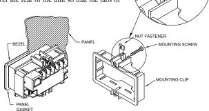
the panel latch engage in the slots on the case. The panel latch should be engaged in the farthest forward slot possible. To achieve a proper seal, tighten the latch screws evenly until the unit is snug in the panel (Torque to approx. 28 to 36 in-oz [0.202 to 0.26 N-m]). Do not over-tighten the screws.
