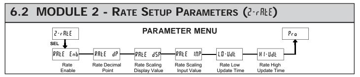
Module 2 is the programming for the rate parameters. For maximum input frequency, Rate Enable should be set to MD when not in use. When set to MD, the remaining rate parameters are not accessible. The rate value is shown with an annunciator of "P" in the Display Mode.
