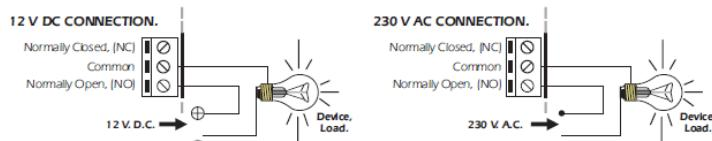
**INFORMATION ABOUT THE OUTPUT.** During the operating mode and according to its load, it could happen a fluctuation or an incorrect working of the output. In such case, you have to install an anti-spark circuit (100 nF/400V Capacitor type X2 and 47 . ½ W resistor) between both contacts of the used relay, as it is indicated on the drawing.
