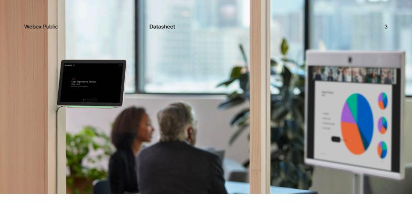
Above: Webex Room Navigator unit mounted on wall
