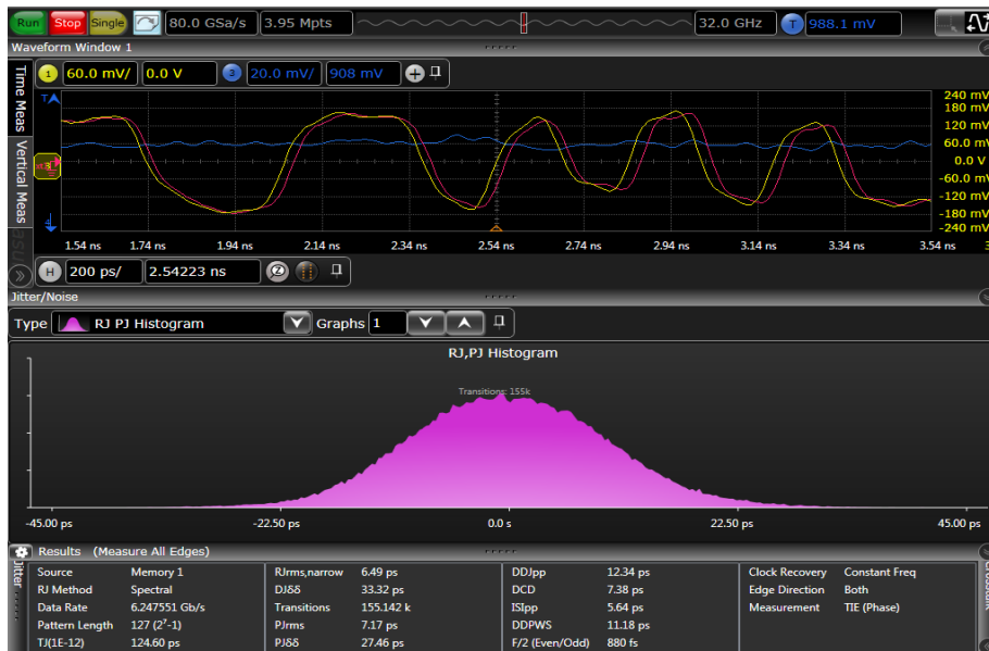
Figure 13. Jitter analysis results using EZJIT, demonstrating the improvement in jitter statistics after removing the jitter generated by the power supply.
