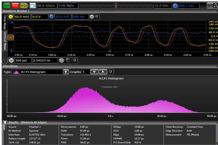
Figure 12. Jitter analysis results using EZJIT, showing the large amount of jitter in the original serial
