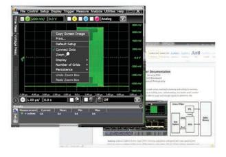
Save information about the oscilloscope, waveform screen captures, and measurement result in one organized report file (PDF or MHTML) to archive and keep proof of test results.
