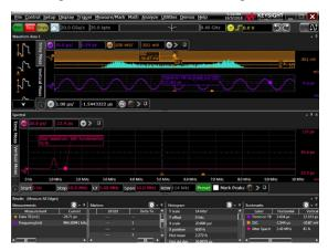
Finally, EZJIT Complete will allow you to make phase noise measurements on clock signals. Keysight is the first to offer a dedicated phase noise measurement application on Infiniium oscilloscopes. Phase noise is related to clock TIE and is generally used to measure change in an oscillator's frequency, either in the long term or short term.
