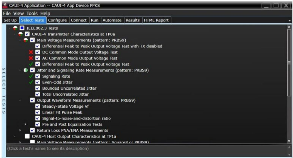
Figure 2. The Keysight automated test engine quickly guides you through selecting and configuring tests, setting up the connection, running the tests, and viewing the results. You can easily select individual tests or groups of tests with a mouse-click.
