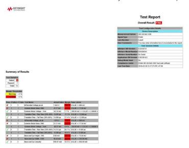
Figure 5. The OIF-CEI 4.0 compliance test application software results screen shows a summary of the tests performed, pass/fail status, and margin. Hyperlinks direct you to the more details of that test.
