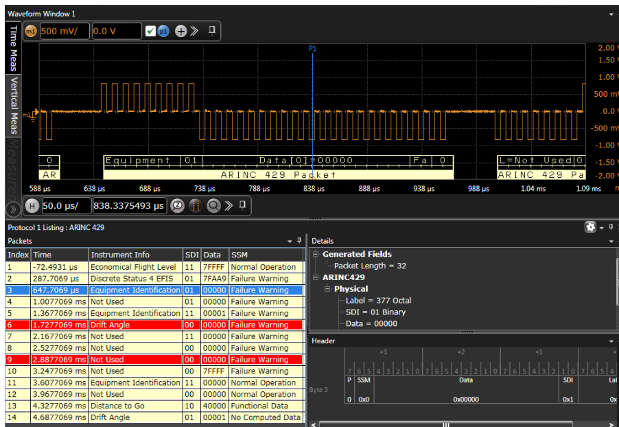
Figure 1. Protocol decoding of ARINC 429 showing a real time trace, protocol decoding table, and packet details using a symbolic decode.
