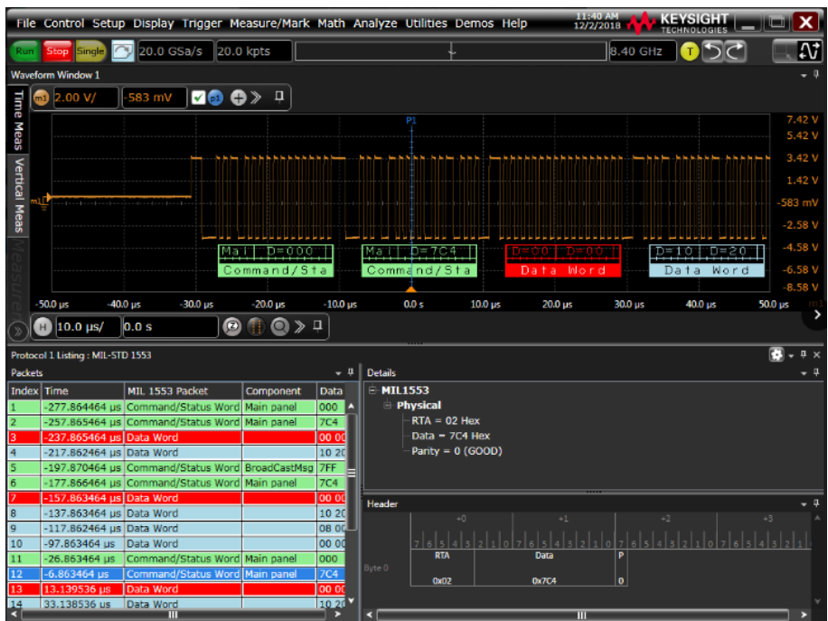
Figure 2. Protocol decoding of MIL-STD-1553 showing a real time trace, protocol decoding table, and packet details using a symbolic decode.
